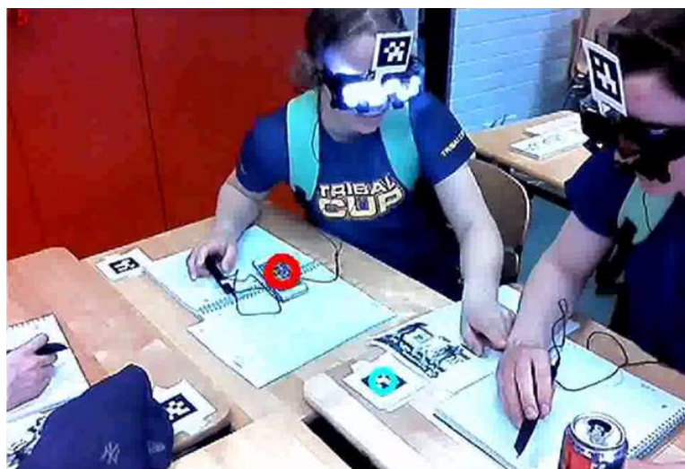
Figure 1. A frame from eye-tracking video showing students wearing the trackers. The red circle indicates the computed location of teacher gaze and the blue circle indicates the visual marker that is closest to gaze target. The bright light around student eyes is infrared, which is invisible to the naked eye.
