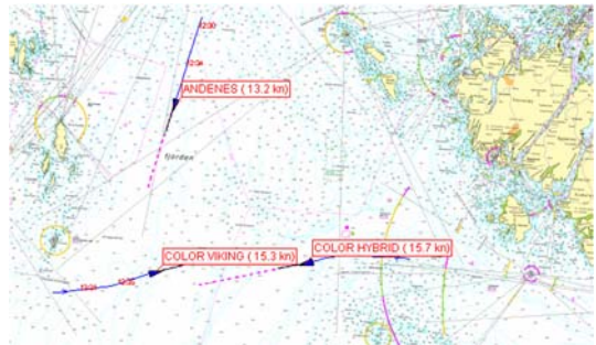
Fig. 4. Encounter in the Oslo fjord. Color Hybrid and Andenes is heading into a close quarter situation. The red dotted heading line in front of each AIS target is an extrapolation of present movement for the next 10 minutes. See text for details. (Screen dump from kystinfo.no 20220509 at 14:38)
