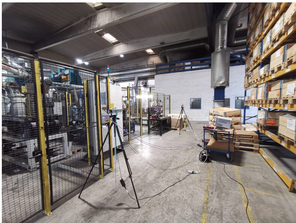
Figure 2. Measurement setup in Manufacturing hall at Dokka Fasteners AS. On the right side, the metallic shelves contain many pieces of heavy-duty equipment inside the wooden boxes. The left side contains many robotic types of machinery surrounded by a metal fence with an metallic alarm box and a grille door.
