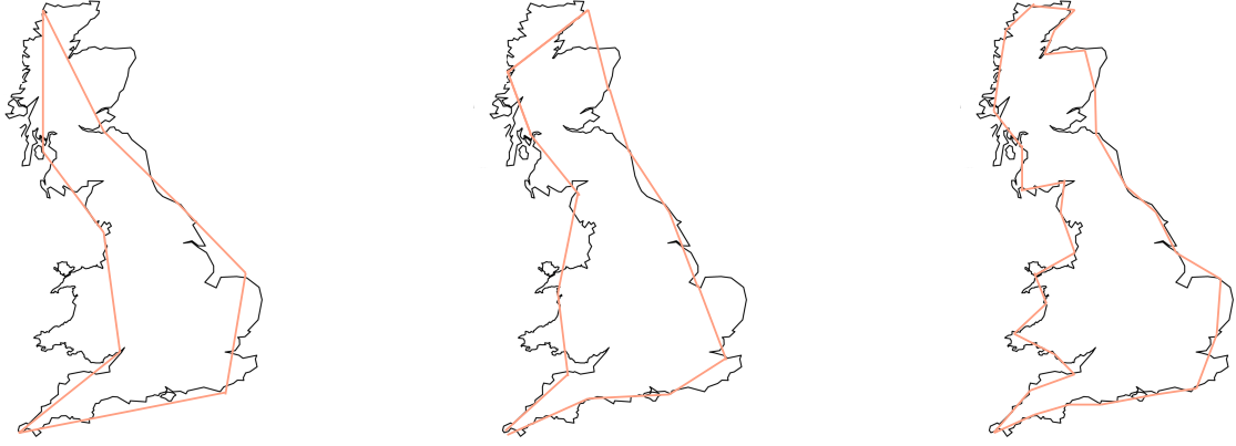
Figure 2.1.: Illustration of Mandelbrot's divider method for measuring the coastline of Britain. By decreasing the divider lengths (orange lines), a more precise reconstruction of the map is achieved. Illustration adapted from Landgraf and Hansmann (2019).
