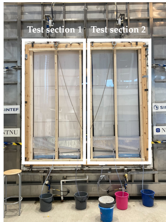
Figure 4. The test rig seen from the interior side. The water-collecting system consists of buckets and tubes. The left side of the rig is test section 1, and the right side is test section 2.
