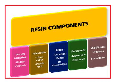
Figure 5. Resin components in stereolithography (SLA) [29].
