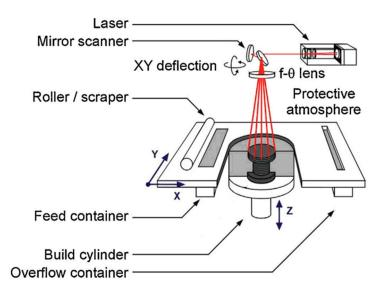
Figure 6. Illustration of SLS process (reprinted with permission) [61].
