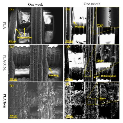
**Figure 7.** Surface morphology of PLA and PLA-based composite scaffolds after one week and one-month immersion in PBS solution [80].
