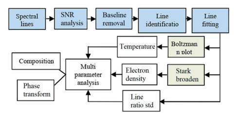
**Figure 8.** Pre-processing and multi-parameter analysis for monitoring of the composition and phase transformation [92].
