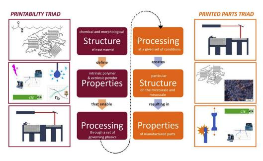
Figure 4. The two, key relationship triads of polymer PBF manufacturing [22].
