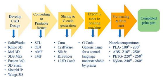
**Figure 13.** Simplified flowchart of FDM process flowchart, representing different types of software employed in the process and suggested nozzle temperature for some materials [96].
