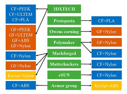
**Figure 12.** Manufacturers of FDM filament and printer (middle column) and their associated fiber-reinforced composite products. Key fibers reinforcements include carbon fiber (CF), glass fiber (GF) and Kevlar (KF), while popular matrixes are nylon, polylactic acid (PLA), PEEK, and acrylonitrile butadiene styrene (ABS) [96].
