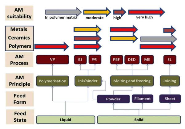
**Figure 10.** A schematic diagram of the relative suitability of additive manufacturing (AM) of three major types of materials (polymers, ceramics, and metals) in various feed forms and states using ASTM processes: Binder jetting (BJ); directed energy deposition (DED); material extrusion (ME); (4) material jetting (MJ); powder bed fusion (PBF); sheet lamination (SL); and vat photopolymerization (VP) [97].
