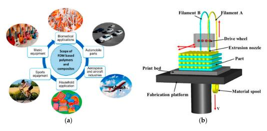
**Figure 3.** (a) Applications of FDM-based polymers and PMCs [12], and (b) schematic representation of a typical FDM setup [14].
