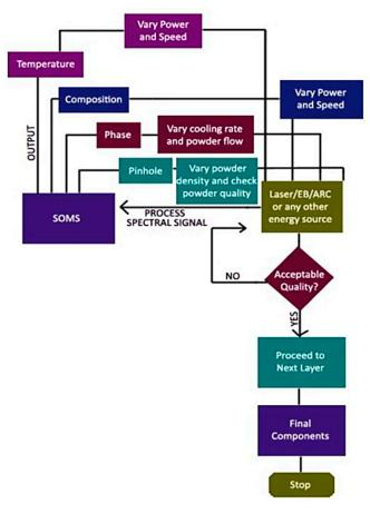
Figure 9. Flowchart for SOMS-based closed-loop control for AM [92].
