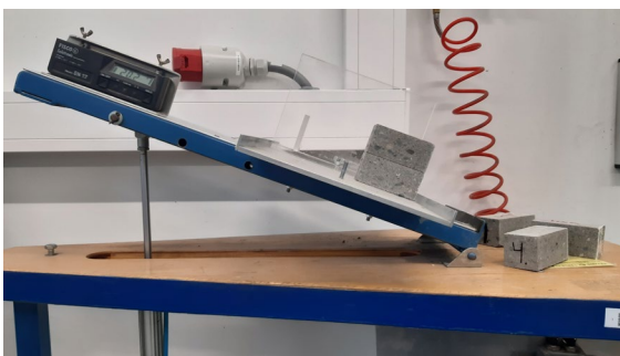
Fig. 6 Test apparatus used for the tilt-tests
