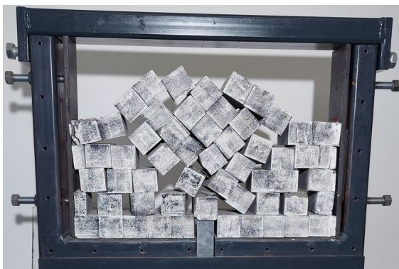
Fig. 15 The model run to failure with 5 layers. The block model failed as an inverted cone
