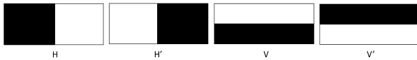
Figure 2: Horizontal and vertical binary patterns and their complements employed with form-factor modulation.
