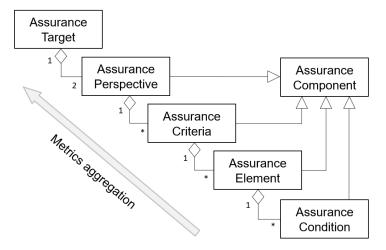
Figure 1. Compositions of the security assurance evaluation model.
