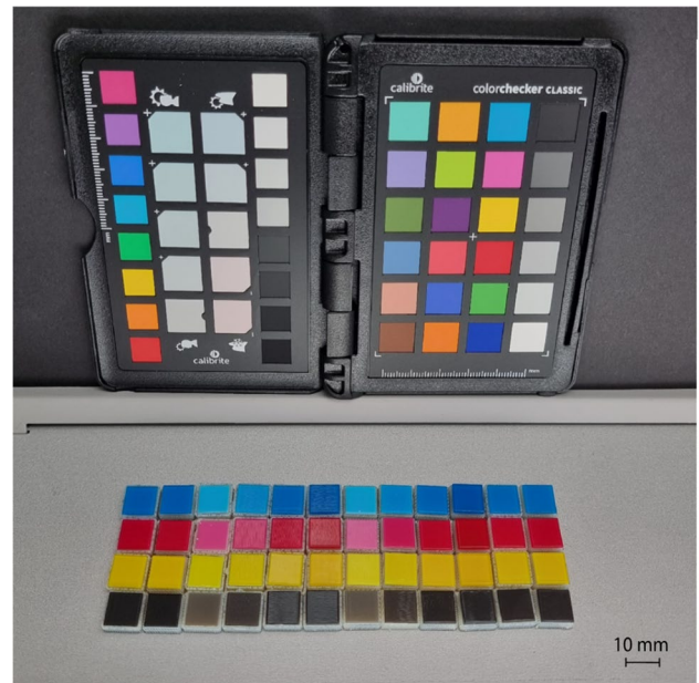
Fig. 2 As-printed MJT samples for color evaluations as observed under D50 daylight illumination
