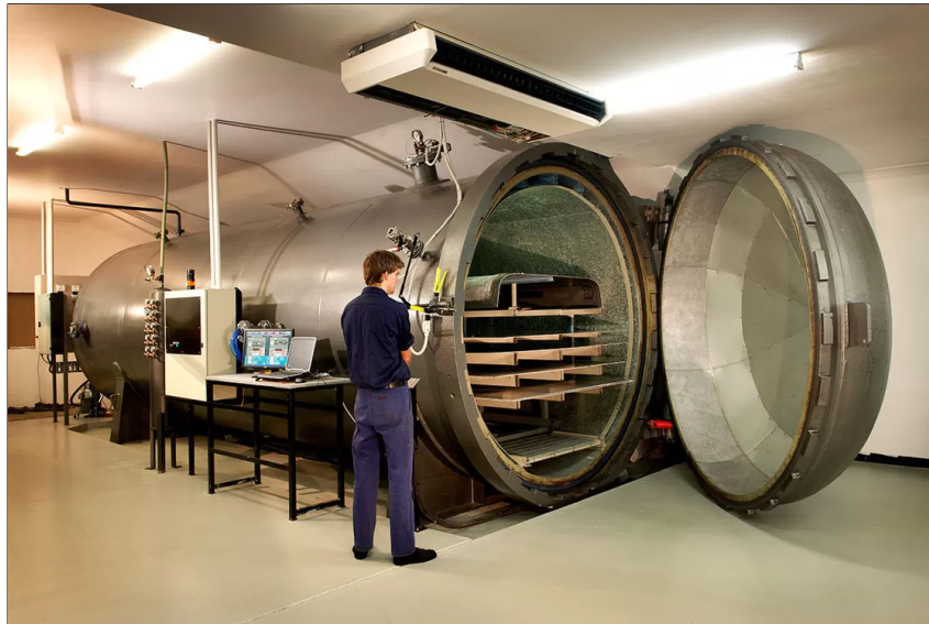
Figure 2.6: Typical industrial autoclave
