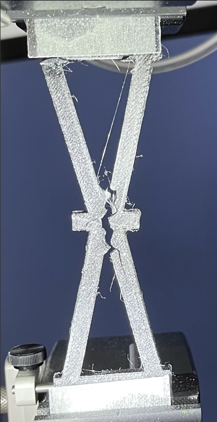
Figure 4.18: Failure mode of reinforced specimen with 30 degree rib angle
