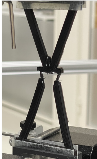
Figure 4.16: Applying stress after failure on reinforced specimen with 45 degrees rib angle
