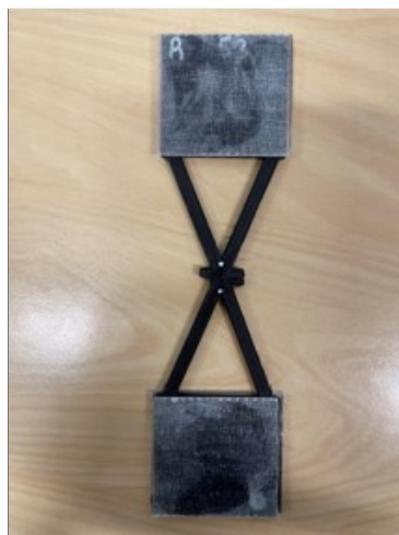
Figure 3.8: Specimen with glass fibre tabs attached
