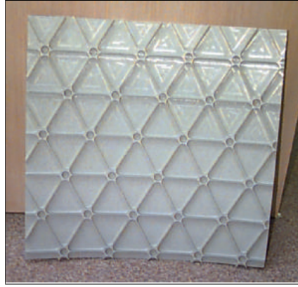
Figure 2.1: Aluminum isogrid panel [15]
