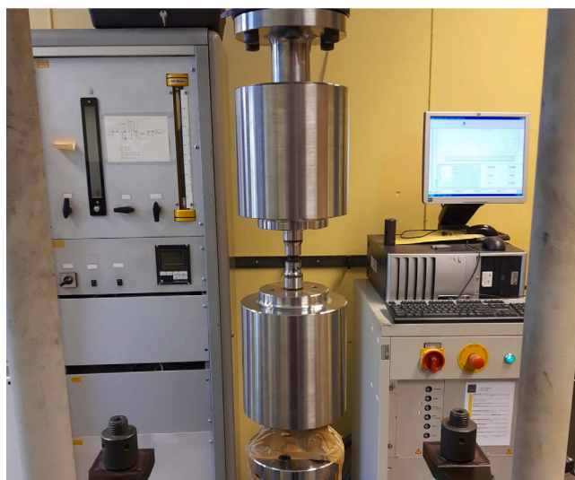
Fig. 4. Fatigue rig for tension loading in TP1. Housings of the spherical bearings that were installed to relieve any bending moment loads are visible.
