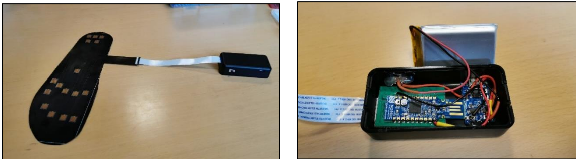
Figure 4. Prototype of the developed insole.
