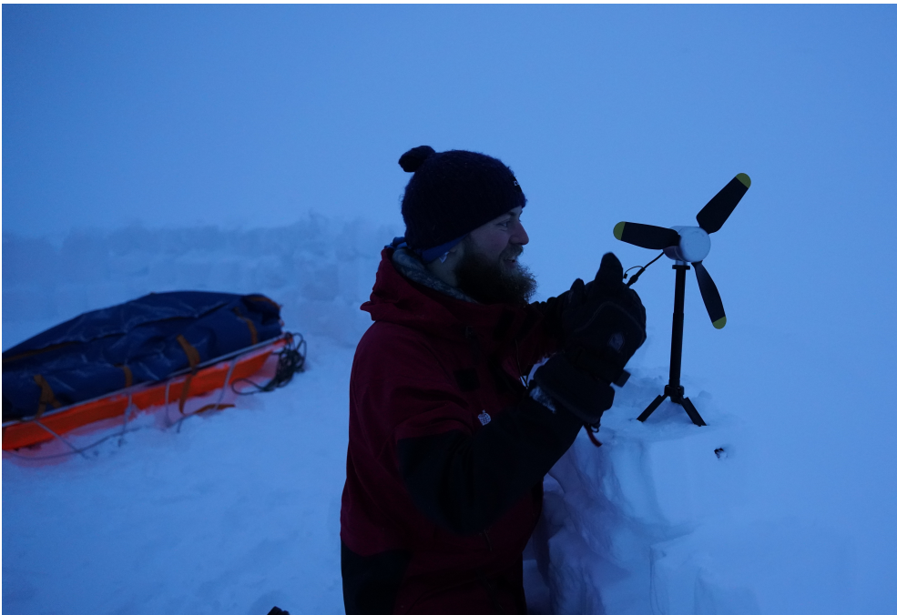
Figure 1: The author investigating the viability of charging small electrical appliances by harnessing the wind power potential near Longyearbyen on Svalbard.
