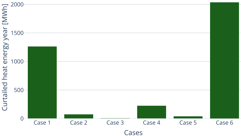
Figure 6.9: The curtailed heat energy for each of the six cases. This energy was recovered from waste heat, but not needed for the district heating system at the time and thus discarded.
