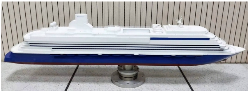
Figure 3.7: Scale model of Vista class cruise ship, used for the wind tunnel experiment by Wang et al. [18].
