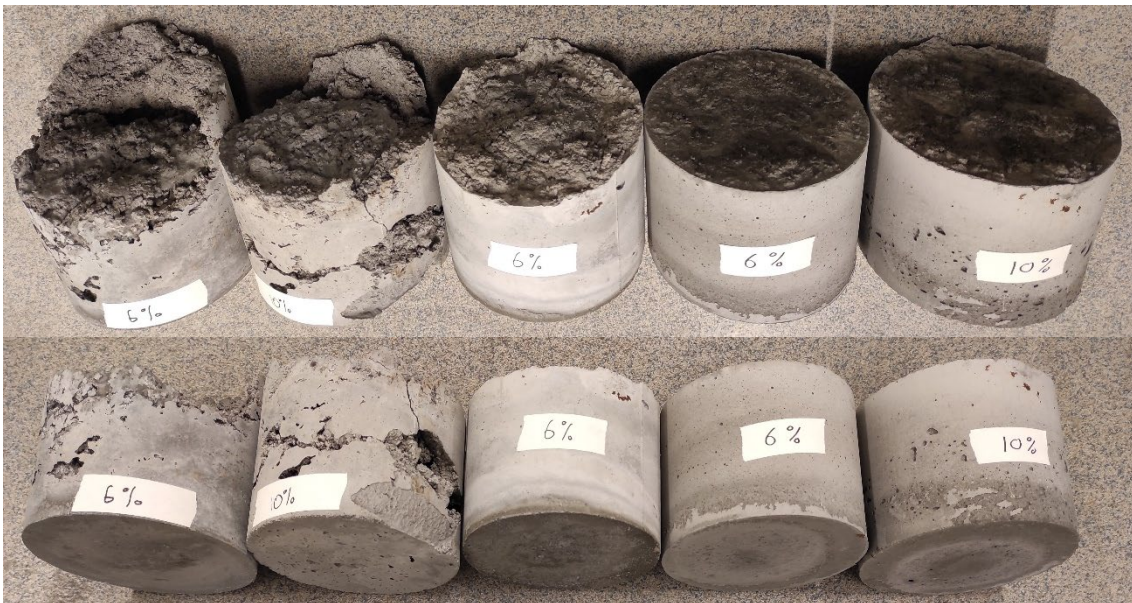
Figure 2 – Cylinders cast during method development – cylinders from early trails are to the left and those from later trials to the right of the photographs.
