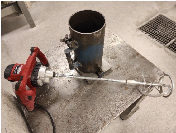
Figure 1 – Hand mixer, 150 mm diameter steel cylinder and vibration table used to mix and cast concrete with set accelerator.
