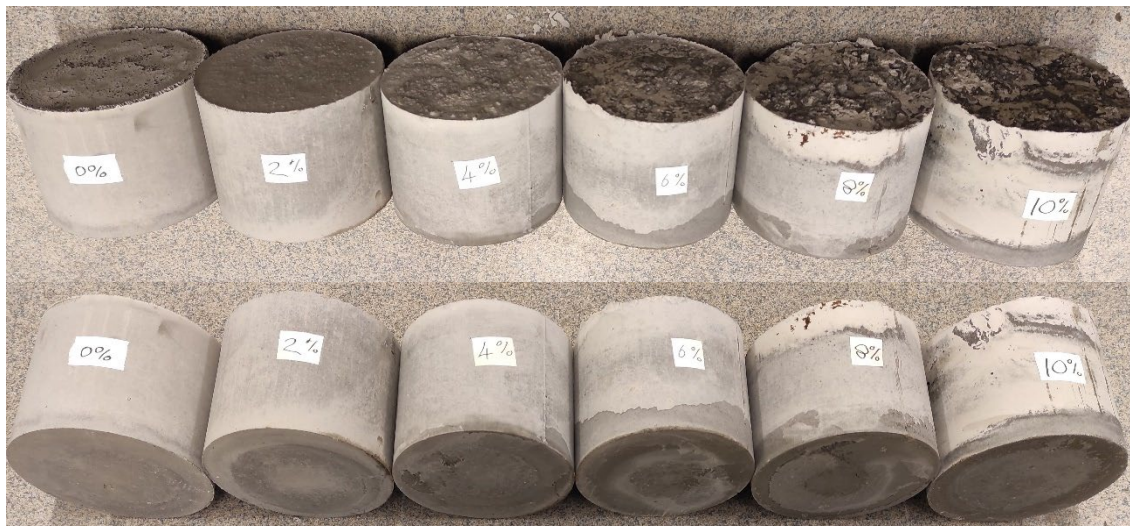
Figure 3 – Cast cylinders with different set accelerator doses
