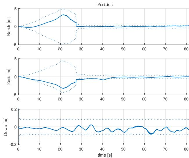
Fig. 8. Estimation error in position in the fourth dataset
