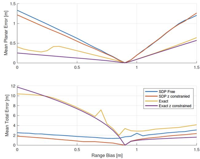
Fig. 12. Re-projection error using elliptical path
