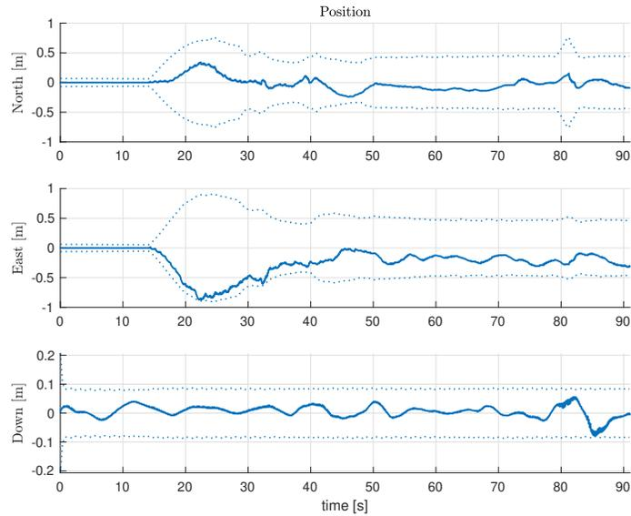
Fig. 5. Estimation error in position in the first dataset
