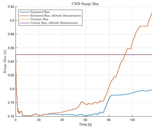
Fig. 19. Estimated UWB bias with virtual altitude measurement in dataset 2
