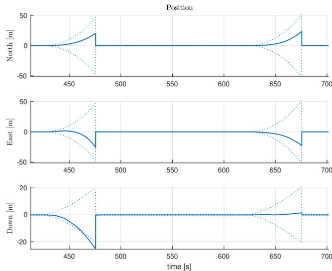
Fig. 9. Estimation error in position during dead reckoning (pure INS without aiding)
