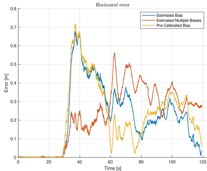
Fig. 17. Error in horizontal position with UWB bias estimation in dataset 2
