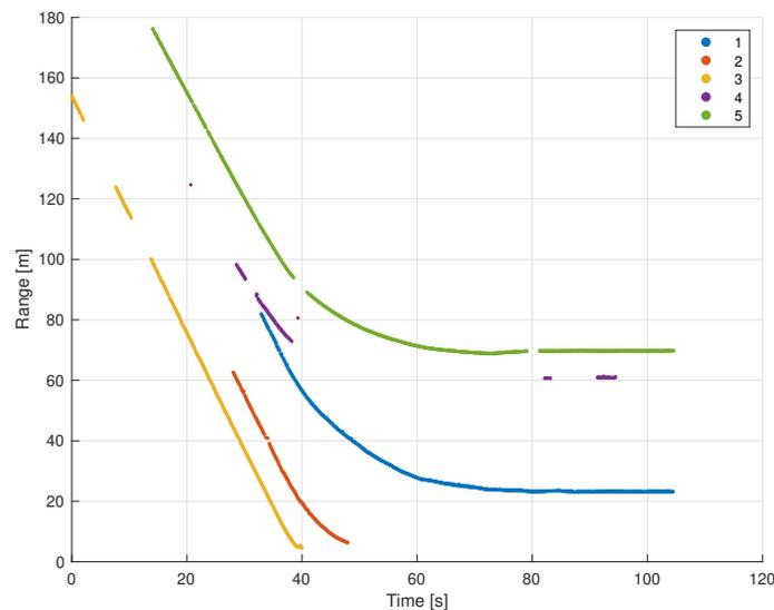
Fig. 3. Measured range between tag and anchors in the first dataset
