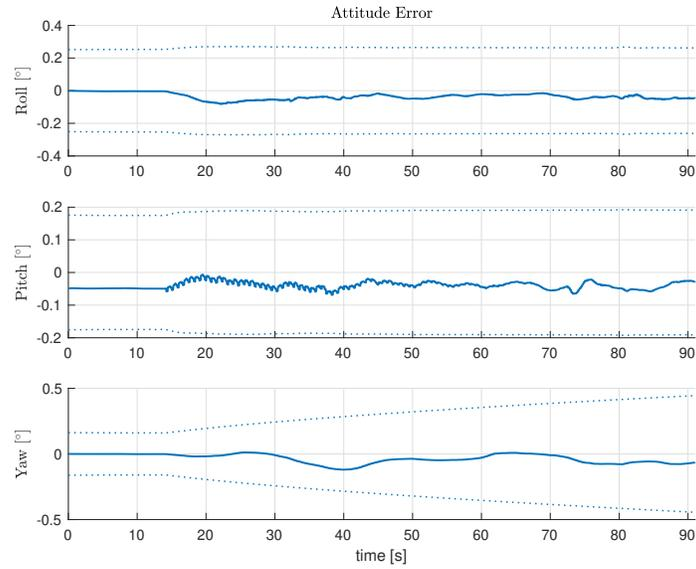
Fig. 7. Estimation error in attitude in the first dataset
