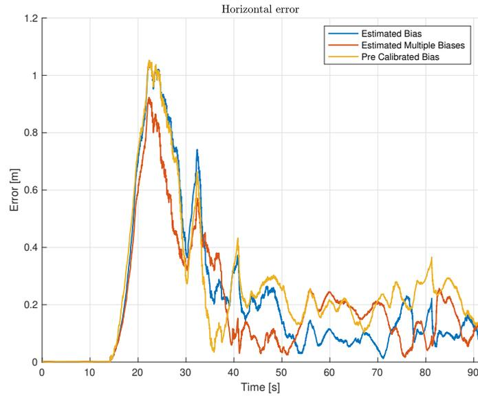
Fig. 16. Error in horizontal position with UWB bias estimation in dataset 1
