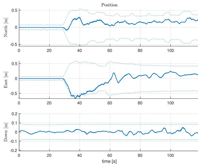
Fig. 6. Estimation error in position in the second dataset
