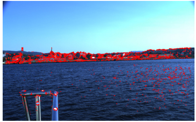
Fig. 5. ORB features detected in an image captured in the open water before arriving at the harbor area.
