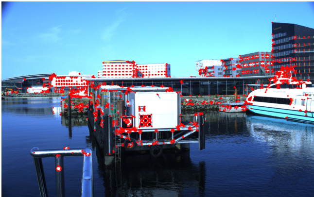
Fig. 4. ORB features detected in an image captured near the docking terminal.
