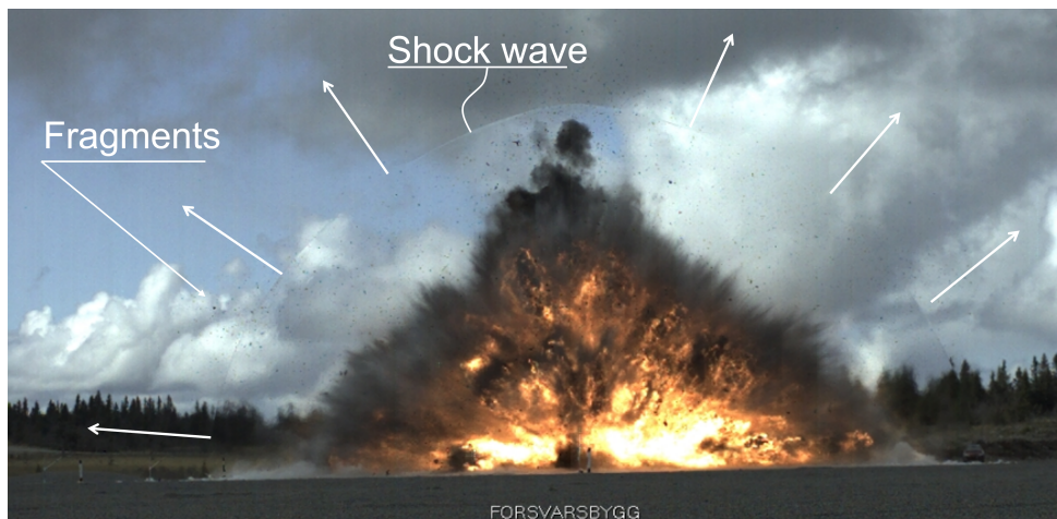
Figure 1.1: Detonation of a vehicle borne improvised explosive device, illustrating accelerated fragments moving together with the shock wave. The propagation of the shock wave is indicated with the white arrows. Courtesy of The Norwegian Defence Estate Agency (Forsvarsbygg).
