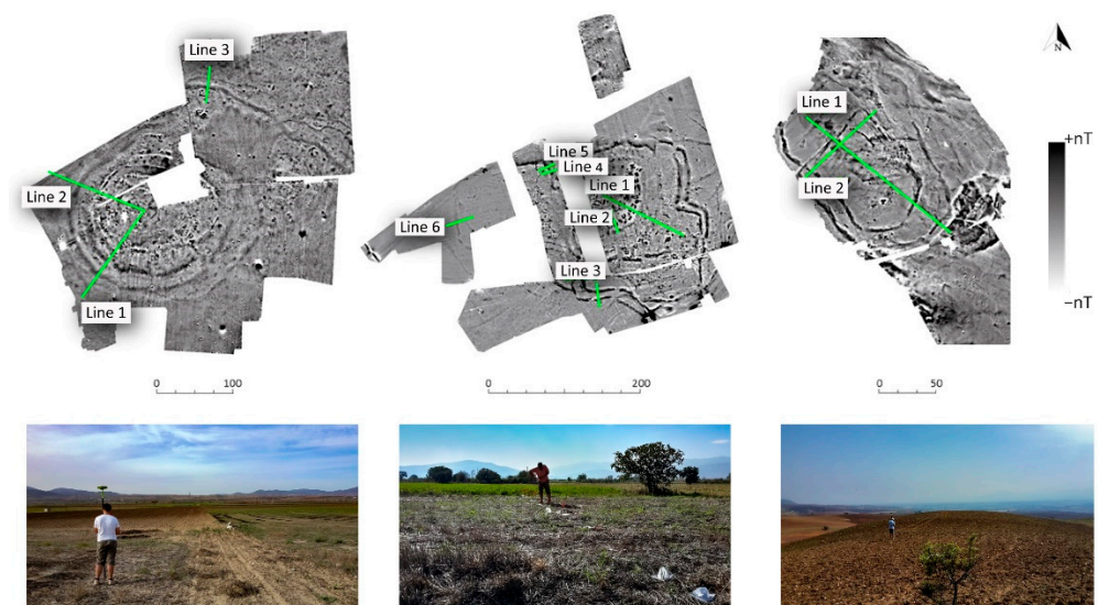
Figure 2. General location of the soil sample lines over the magnetometer results ( top ). General views of the fields during soil sampling ( bottom ). The grayscale image shows positive magnetic anomalies in black and negative anomalies in white.
