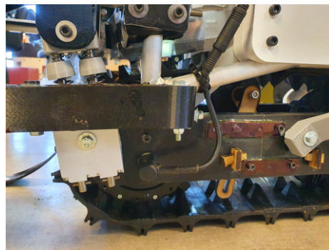
(a) Suspension mounting bracket with fixes. (b) Suspension mounted and lowered on sit-ski.
