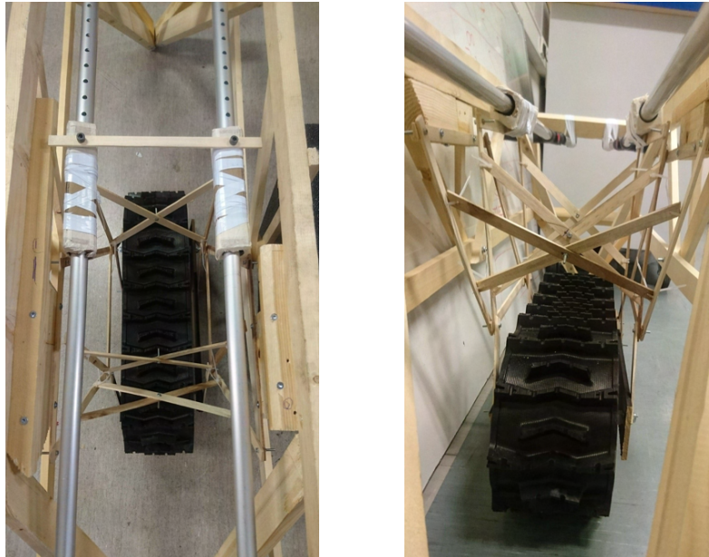
(a) Sliding mechanism for height adjustment with cardboard and crutches mounted on wood chassis, top view (b) Sliding mechanism for height adjustment with cardboard and crutches mounted on wood chassis, inside view
