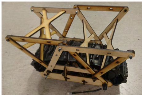
(a) Suspension set-up in laser-cut MDF.
