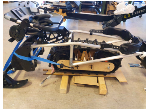
(b) Frame with motor and belt inside frame after two tube members were removed.
