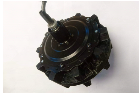
(a) Cardboard cogwheel prototype and reference drawing of cogwheel dimensions. (b) Electric motor with cogwheel made using additive manufacturing.
