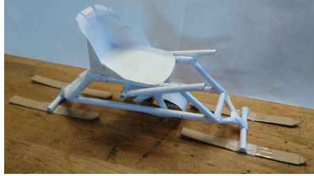
Figure 14: Small size paper model with chassis, four skis, height adjustment mechanism and seat.
