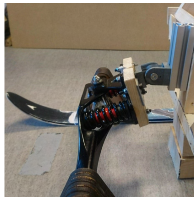
(b) Adjustable steering module lower angle setting
