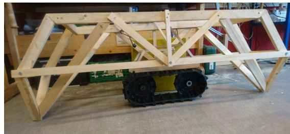
Figure 17: Full size wood chassis frame prototype.
