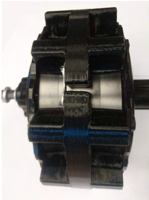
Figure 42: Connection of the two motor cogwheel parts.
