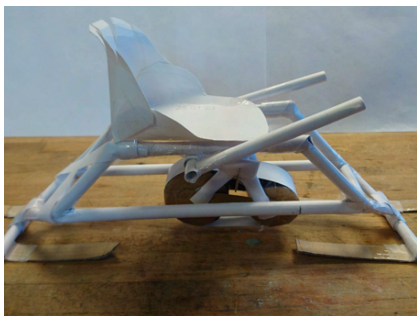
(a) Height adjustment mechanism in lifted position (b) Height adjustment mechanism in lowered position on small scale paper model
