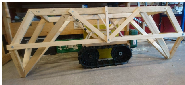
Figure 13: Full size wood chassis frame prototype.
