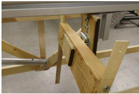
(a) Sliding mechanism with aluminium rails in lower position.
