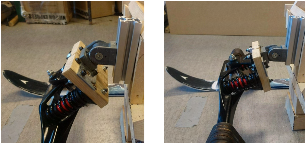
(a) Adjustable steering module higher angle setting. (b) Adjustable steering module lower angle setting.
