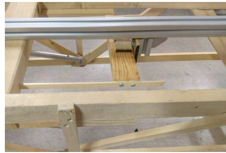
(b) Sliding mechanism with aluminium rails in raised position on wood chassis.
