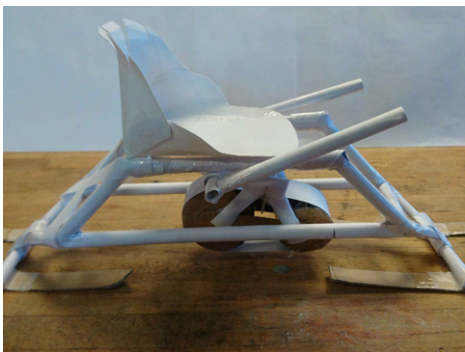
(a) Height adjustment mechanism in lifted position on small scale paper model. (b) Height adjustment mechanism in lowered position on small scale paper model.
