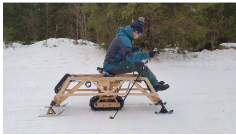
(a) User double poling with motor propulsion assistance on flat ground before small slope.
