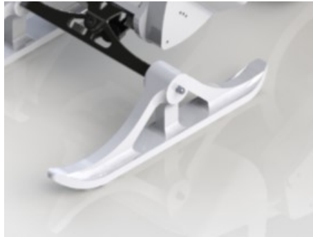
Figure 67: Ski designed in CAD to be 3D-printed.
