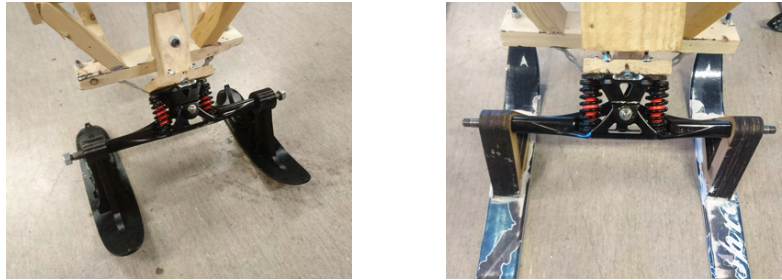
(a) Front steering module with skis on final prototype (b) Rear steering module with skis on final prototype
