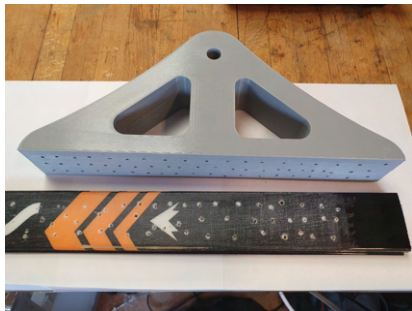
(a) Children ski and binding with drilled holes before glueing.
