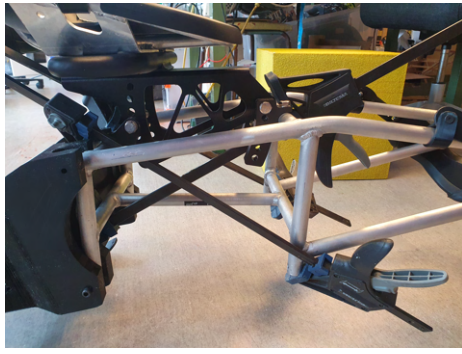
(a) Frame before removal of the two tube members.
