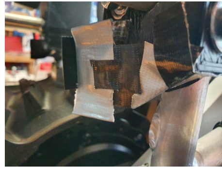
(b) End stopper covered in tape as protection.
