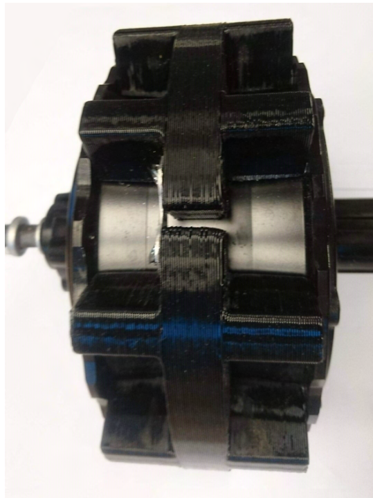
Figure 38: Connection of the two motor cogwheel parts.
