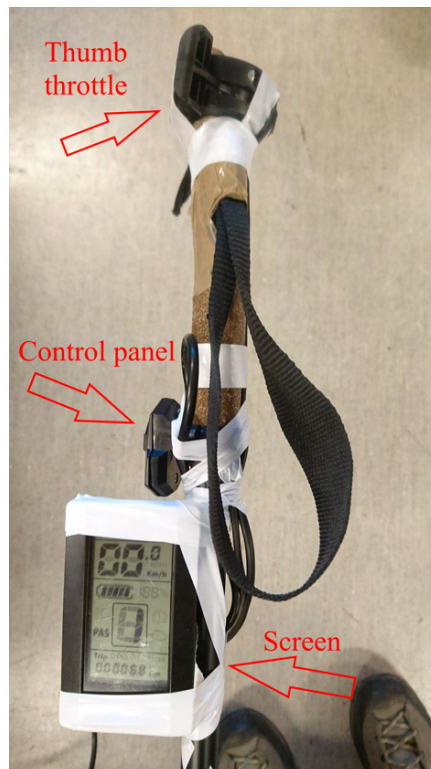
Figure 31: Motor control unit on ski pole.
