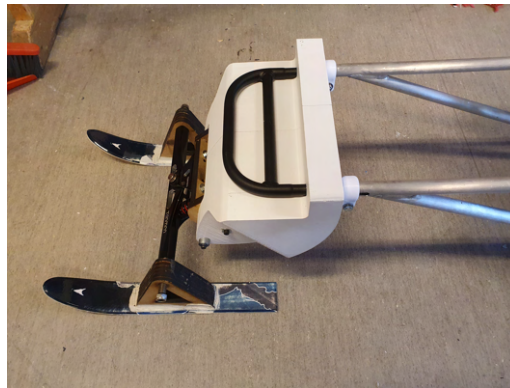
Figure 56: New front steering module on the Exero Spike Snow frame.
