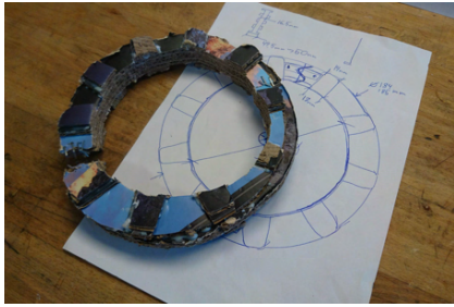
(a) Cardboard cogwheel prototype and reference (b) Electric motor with cogwheel made using additive manufacturing
