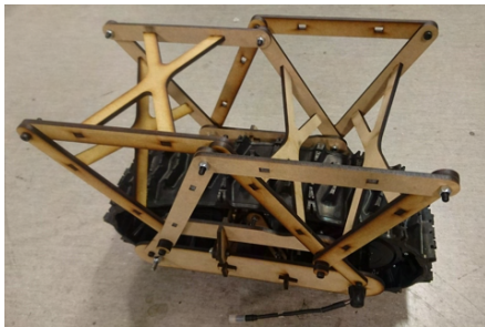
(a) Suspension setup in laser cut MDF
