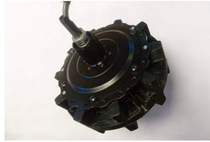
(a) Cardboard cogwheel prototype and reference (b) Electric motor with cogwheel made using additive manufacturing
