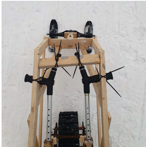
Figure 40: Steering module not mounted perfectly straight on chassis.
