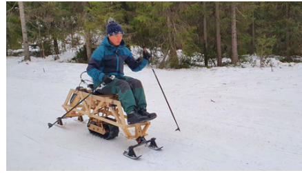
(b) CCSS with user leaning to the left to maintain straight forward travel down small slope
