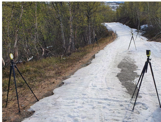
Figure 95: Picture of the flat section with timing equipment on the side creating gates.
