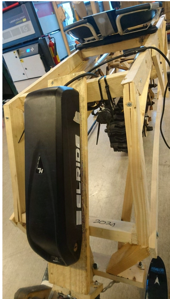
Figure 36: Battery mounted at the rear of the chassis with cables attached to chassis.
