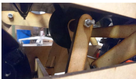
(c) Belt tension mechanism with wheel inside suspension module.
