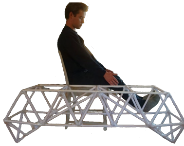
Figure 16: Full size paper model of chassis with user sitting on chair behind to test sitting position and general form.
