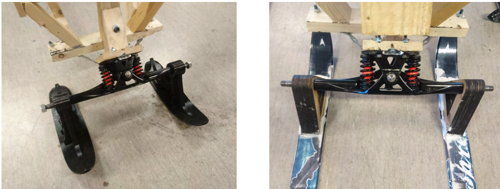
(a) Front steering module with skis on final pro- (b) Rear steering module with skis on final proto- type. type.
