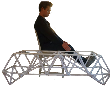
Figure 12: Full size paper model of chassis with user sitting on chair behind to test sitting position and general form.
