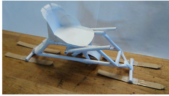
Figure 10: Small size paper model with chassis, four skis, height adjustment mechanism and seat.
