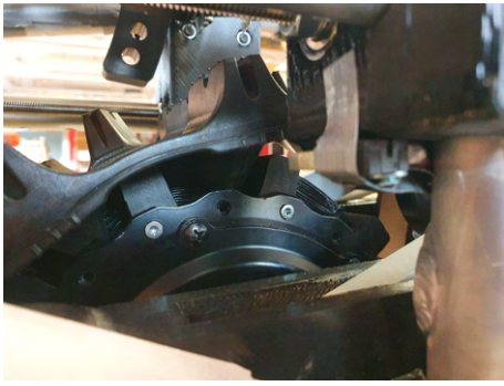
(a) End stopper before tape as protection.
