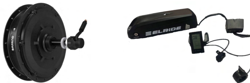
(a) Bafang RM G040.250.D 36V 250W electric bicycle hub motor (b) Battery with wiring and motor control unit with control panel and screen in centre and thumb throttle for speed regulation in bottom right
