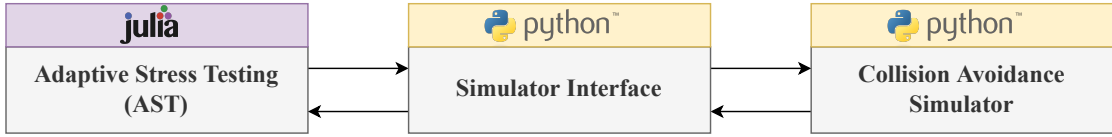
Figure 3.2: Maritime Adaptive Stress Testing. In this figure, an abstract overview of the MAST architecture is shown. Two different programming languages are used; the simulator provided by Zeabuz is implemented in Python, and the AST-framework, developed by NASA, is implemented in Julia. In between, we have the simulator interface developed in this work and implemented in Python, which helps the communication between the AST software package and the simulator. The arrows indicate communication between the parts.
