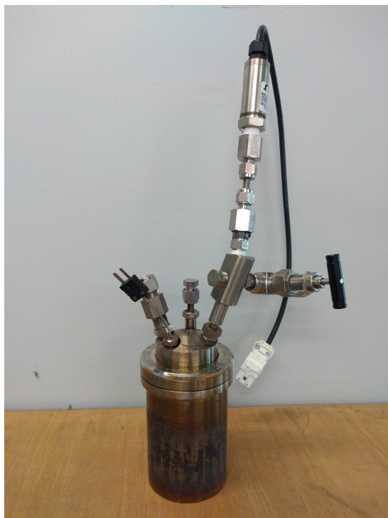
Figure 3.3.1: The stainless steel reactor used for synthesis of silicon nanowires.
