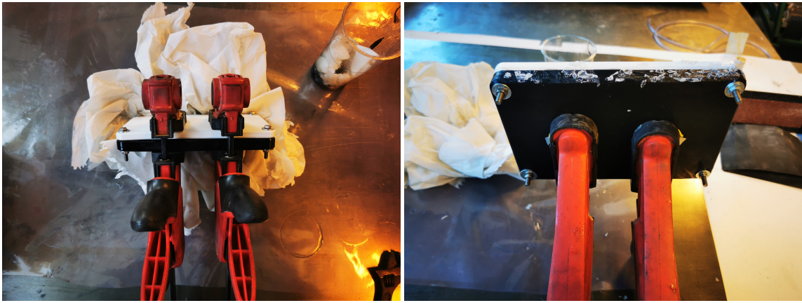
(a) The mold bolted and clamped shut.
