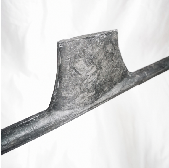
(c) The finished forging of the fuselage showing the flange transition at the front.
