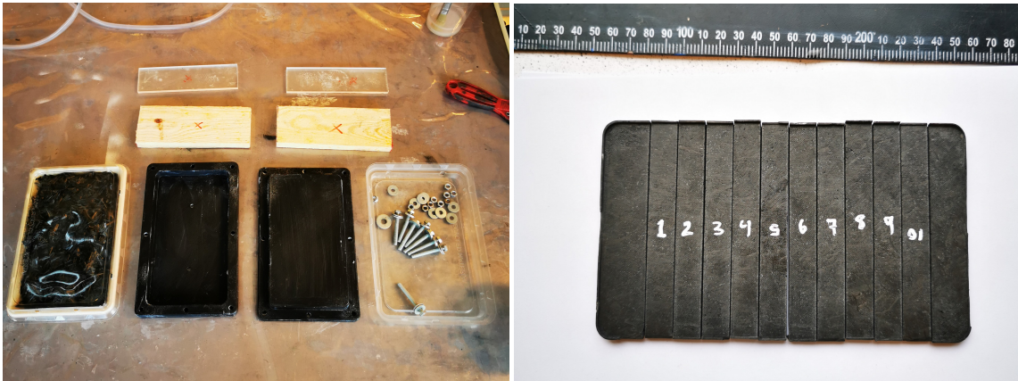
(a) The materials used for the second batch of test specimens. (b) The batch 2 test specimens after being cut with the water jet..
