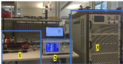
FIG. 11. Measurement instruments. The setup consisted of the lamination test sample (1), the power analyzer, YOKOGAWA WT3000 power analyzer (2), and the power supply, ITECH IT7627 high power programmable AC power supply (3).
