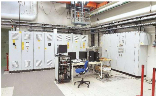
FIGURE 2 Test circuit (transformer winding connection and dc-bias implementation) and the EGSTON grid emulator (controllable three-phase voltage source) in the National Smart Grid Laboratory (NSGL), Norway
