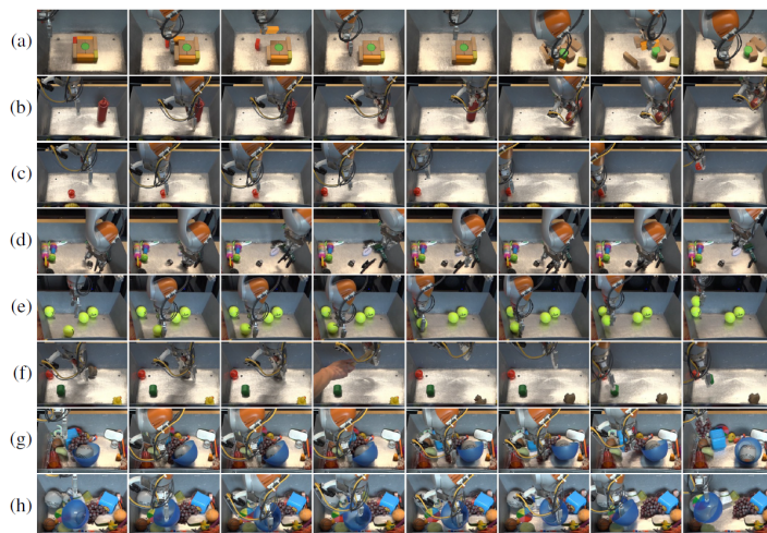
Figure 2.6: Eight grasps from the QT-Opt policy, illustrating some of the strategies discovered by their method: pregrasp manipulation (a, b), grasp readjustment (c, d), grasping dynamic objects, and recovery from perturbations (e, f), and grasping in clutter (g, h). (credit[15])
