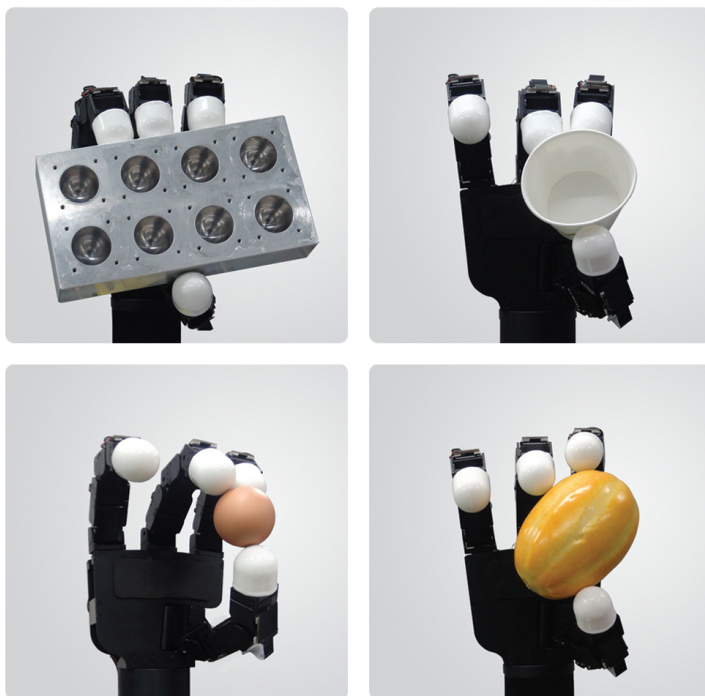
Figure 2.1: The Allegro Hand. (Image is from wiki.wonikrobotics.com .)
