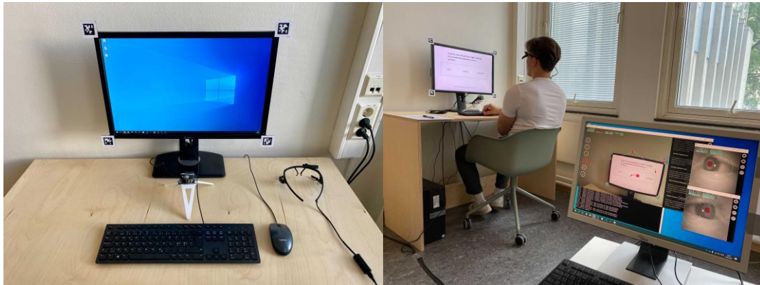
Figure 2. Left) Monitor with apriltags, Pupil Core to the right, and microphone in the middle. Right) Experimenter monitors eye-tracking real time during experimental run.
