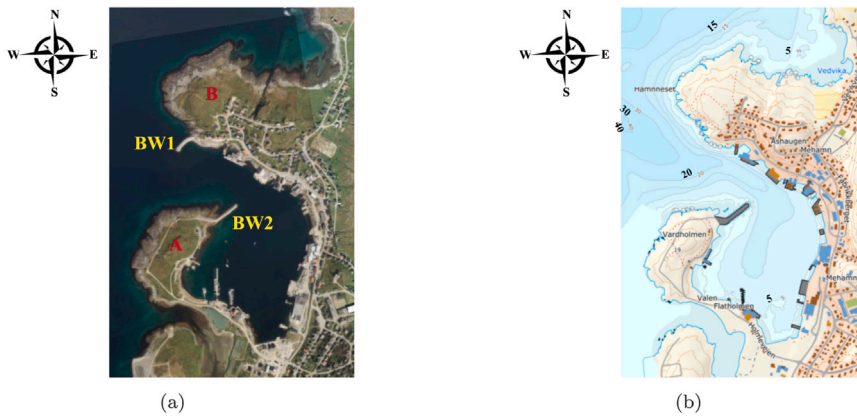
Fig. 26. Mehamn harbour: (a) satellite image; (b) water depth contour. The two breakwaters are marked as BW1 and BW2 and the two peninsulas are marked as A and B.
