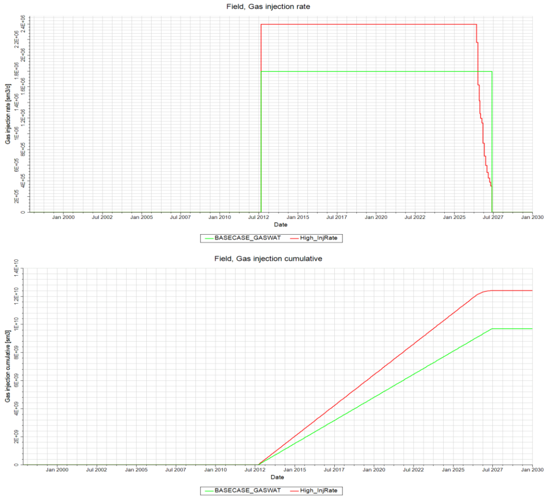
Figure 7-24 (top) Field Gas injection rate (bottom) Cumulative gas injection for the sensitivity of high injection rate case.
