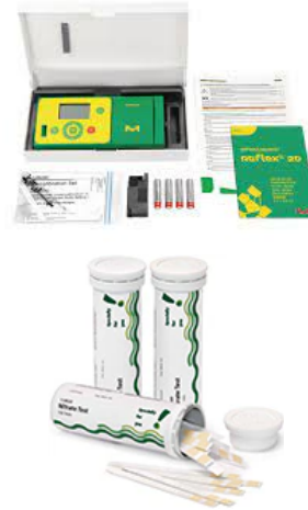
Figure 3.24: The Merck Reflectometer RQflex® 20 (top) was used to make glucose and lactate measurements from the bioreactor samples. The RQflex® 20 can be programmed with little strips to make optical measurements of both glucose and lactate from a liquid sample. The glucose and lactate test strips arrive in little vials (bottom).
