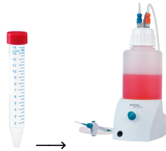
Figure 3.19: Trypsin was sucked out of a centrifuged falcon tube, leaving the cells in a pellet at the bottom side of the tube. The falcon tube was brought back inside a LAF bench and a Integra Vacusafe lab Aspiration System was used to suck out the trypsin.
