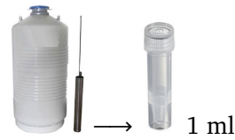
Figure 3.4: A liquid nitrogen storage container (left) used to freeze and store cells for biotechnological experiments. The MuSC were kept in such a container, protected from icicles with freezing media inside vials (right).
