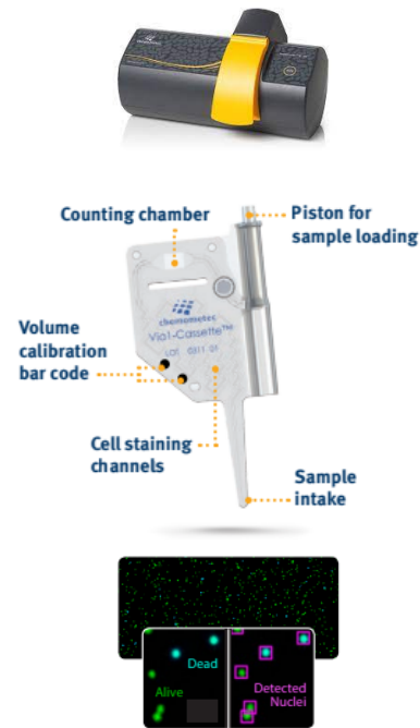
Figure 3.21: NucleoCounter® NC-202™ (top) from ChemoMetec with an accompanying Via2-Cassette™ (middle). Samples can be taken with the cassette and then be used to measure cell quantity with the NucleoCounter® machine and ChemoMetec's PC software (bottom).
