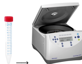
Figure 3.18: The falcon tube was centrifuged for 5 minutes at 550 RPM.
