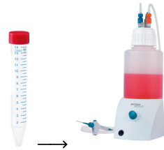
Figure 3.8: Cryogenic media can be sucked out of a centrifuged falcon tube, leaving the cells in a pellet at the bottom side of the tube. The falcon tube was brought back inside a LAF bench and a Integra Vacusafe lab Aspiration System was used to suck out the cryogenic media.
