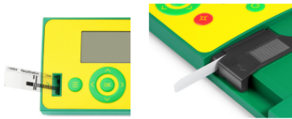
Figure 3.25: The reflectometer is calibrated and programmed to make various measurements with a bar code strip, inserted into the bar code scanner on the front face of the machine (left). Once programmed, a sample test strip which has been immersed into a sample (or calibration strip during recalibration) can be inserted into the strip adapter (right). Easy to follow instructions on how to operate the machine are presented the screen of the reflectometer and in the user manual (Merck, 2017).
