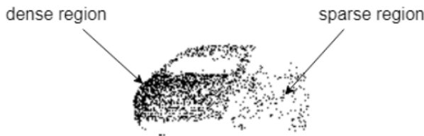
Figure 3.1.: Irregularities of points on a car model produces dense and sparse areas of points. Figure is from [32].
