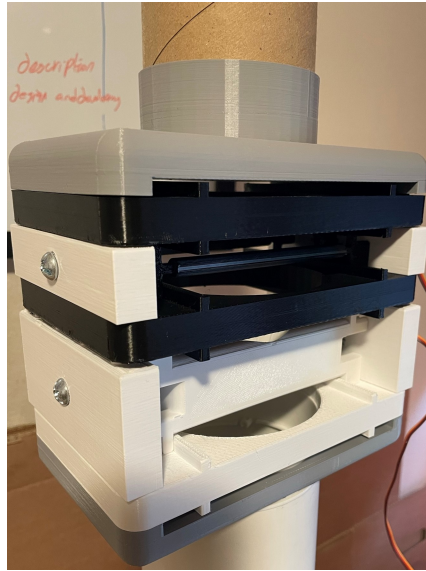
Figure 56: Final Prototype Release Mechanism
