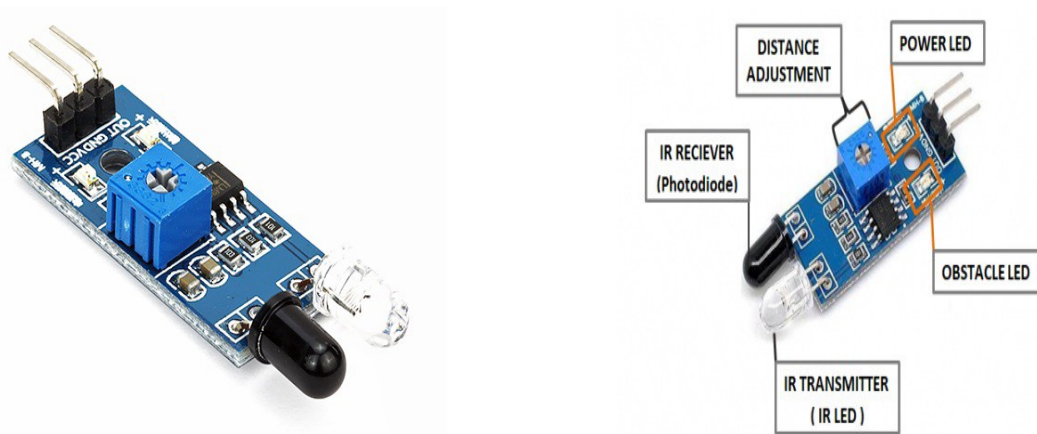
Figure 18: Third Sensors: Infrared Obstacle Avoidance Sensor
