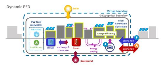
**Figure 2.** Dynamic PED, principle and system boundaries. Including energy efficiency measures, renewables (solar, PV, wind, biomass, geothermal, small hydropower), waste heat recovery, electric and thermal storage, integration of mobility energy needs (and EVs as batteries), sector coupling between electric and thermal, and exchange with the surrounding systems.
