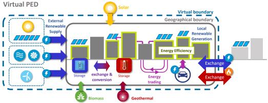
**Figure 3.** Virtual PED, principle and system boundaries. Including virtual integration of external renewables and exchange with the surrounding systems. Including energy efficiency measures, renewables (solar, PV, wind, biomass, geothermal, small hydropower), waste heat recovery, electric and thermal storage, integration of mobility energy needs (and EVs as batteries), sector coupling between electric and thermal, and exchange with the surrounding systems.
