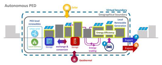
**Figure 1.** Autonomous PED, principle and system boundaries. Only exports to the surrounding system. Including energy efficiency measures, renewables (solar, PV, wind, biomass, geothermal, small hydropower), waste heat recovery, electric and thermal storage, integration of mobility energy needs (and EVs as batteries), sector coupling between electric and thermal.
