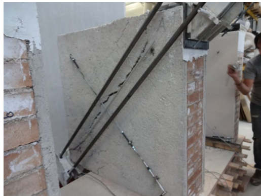
Figure 29. Diagonal compression testing of masonry walls with thermal TRM.
