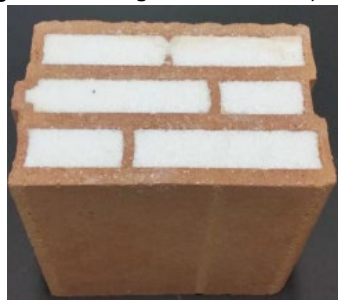
Figure 42. Aerogel-filled masonry units.
