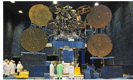
(b) A picture of the satellite Viasat-1 with a mass of 6700kg. https://www.viasat.com/space-innovation/satellite-fleet/viasat-1/
