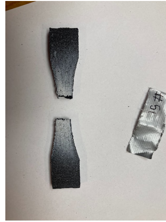
(b) Showing the fracture of specimen nr. 51.
