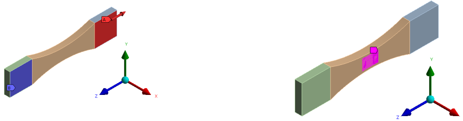
(a) Showing the placement of the 5kN force, section A, and the fixed support, section B, on the vertical validation simulation.
