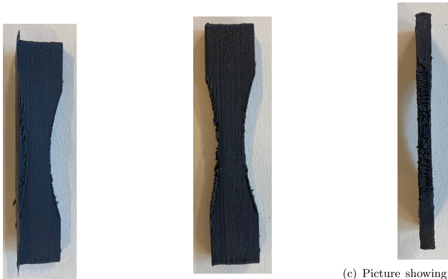
(b) Picture showing how the horizontal rotated samples looked after the removal of the support structure.
