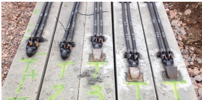
Fig. 5. A type of driven precast concrete energy pile with pipes at the side-walls [32].
