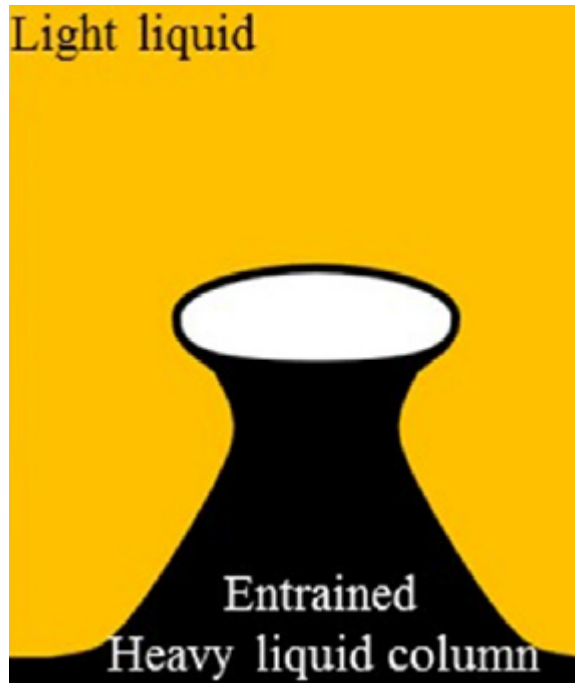
Figure 3: A bubble, passing an interface and entraining the heavy phase [1].
