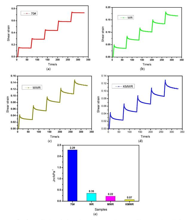
**Figure 5.** Effect of repeated loading-unloading cycles on shear strain and non-recoverable creep compliance (**e**) of virgin asphalt (**a**), WR modified asphalt (**b**), MWR modified asphalt, (**c**) and KMWR modified asphalt (**d**).
