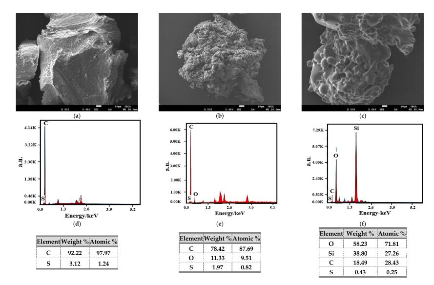
Figure 8. SEM images (a–c) and element distribution (d–f) of the three kinds of waste rubber powder.
