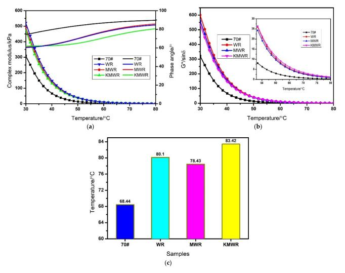
**Figure 4.** Effect of temperature on complex modulus and phase angles (**a**), rutting factor, (**b**) and failure temperature (**c**) of the four kinds of asphalt.
