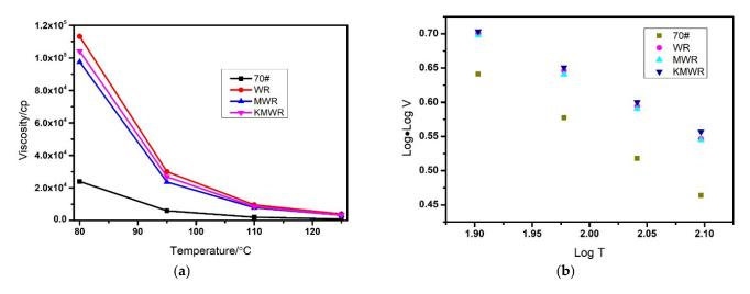
Figure 3. Effect of temperature on viscosity-temperature curves (a) and Log relation (b) of the four kinds of asphalt.
