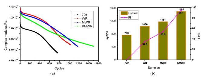
Figure 6. Effect of loading cycles on complex modulus (a) and fatigue life (b) of the four kinds of asphalt.
