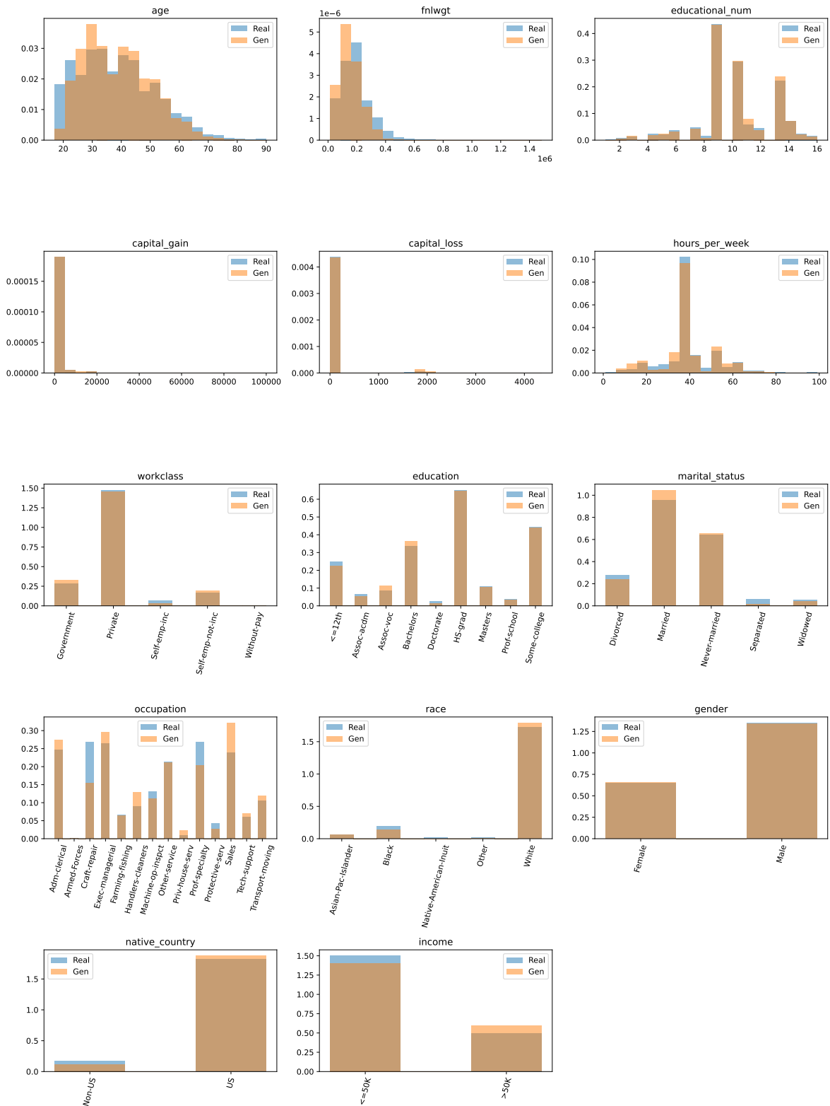
Figure C.5: Histograms of generated samples from TVAE-mod plotted against histograms of observations from the Adult training dataset. One histogram for each column. The synthesized dataset is of the same size as the Adult train dataset.
