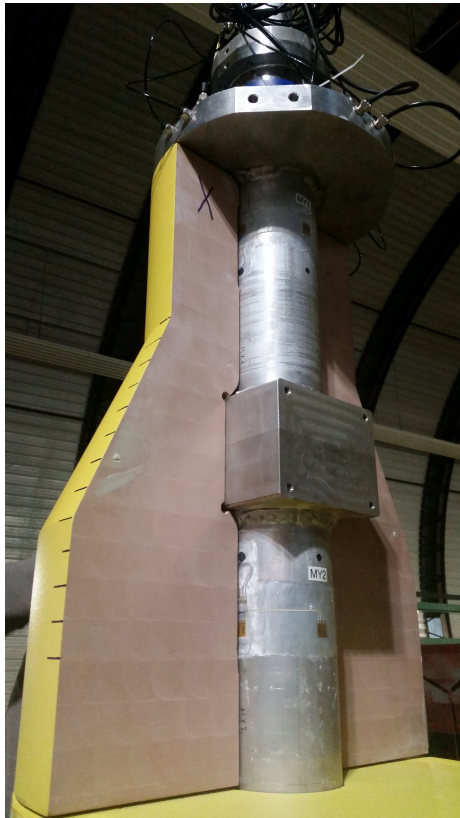
(a) Spar top before the last floater was mounted. The strain gauges are visible on the aluminium backbone.
