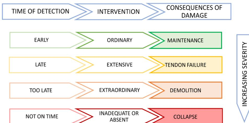
**Figure 3.1.1.** Illustration of typical relationships between how early the damage was detected, the typology and suitability of the interventions carried out, and the structural consequences in terms of increasing severity.
