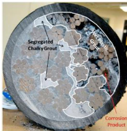
**Figure 4.2.2.5.** Grout segregation appearance (Lau et al, 2016).
