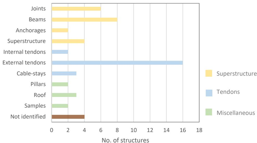
**Figure 3.3.1.** Failure location in the studied structures.
