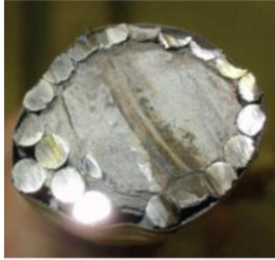
**Figure 2.3.2.** Sorell Bridge (ID-3). Cross sectional view of one of the most severely corroded tendons. The tape just visible around the outside was applied during recovery to keep the tendon together at the cross sectional cut. There is no tendon duct (Papè and Melchers, 2011).
