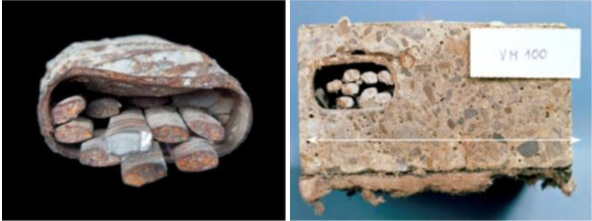
**ID-19.7.** Prestressing wires are almost not embedded in the protective grout (left) or insufficient grouted (right). Only one broken wire (left) shows a non-corroded brittle broken fracture surface. (Helmerich and Zunkel, 2014).
