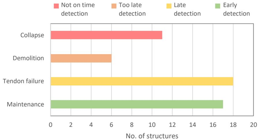
**Figure 3.1.2.** Level of damage of the studied structures.
