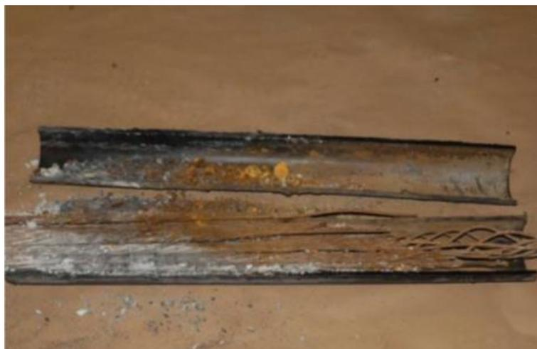
ID-15.3. Segment of failed tendon discovered in January 2011 with evidence of corrosion damage. Duct opened in laboratory during investigation (Ahern et al, 2018).
