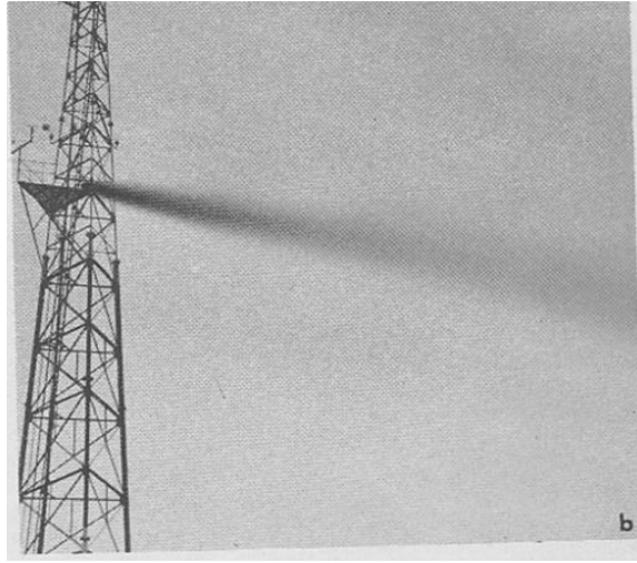
Figure 2.3.5: A continuous emission source captured at 5 minutes of exposure at the Big Rock Point reactor site [5].
