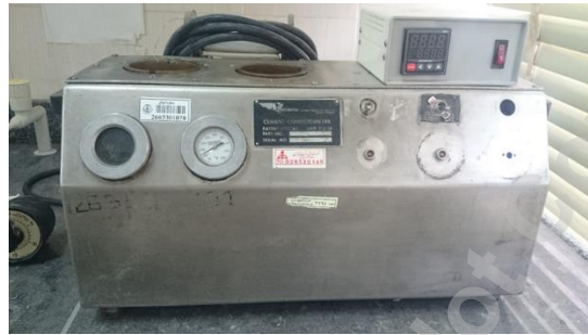
Figure 2. Schematic of a cement consistometer
