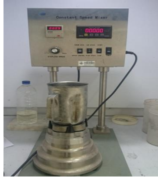
Figure 1. Schematic of a cement slurry mixer
