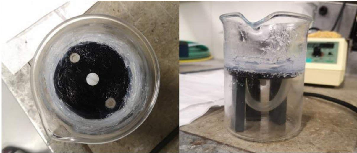
Figure 2.2: The prototype for an artificial burrow shown from the top and the side, consisting of a lightproof plate as 'sediment' and a silicone tube as an artificial burrow. Image: Håkon Sæther
