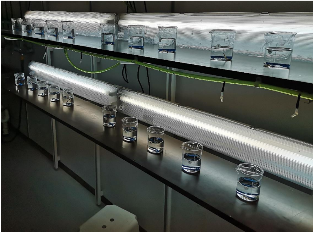
Figure 2.4: The main feeding experiment setup, with the 20 beakers evenly distributed along the top and bottom shelf. Image: Håkon Sæther
