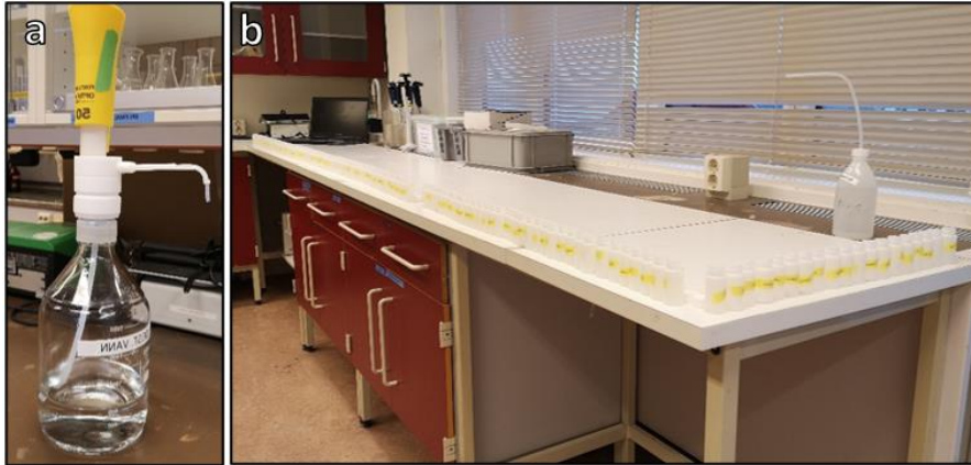
Figure 2.7: a) Optiflex dispenser used for chemical dosing of distilled water and oxidizing agent; b) row of all polyethylene bottles containing filters for particulate phosphorus. Image: Håkon Sæther
