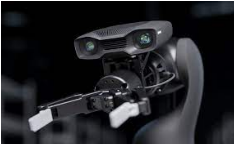
Figure 1: The Zivid Two camera mounted on a robot arm (Borgan 2022).
