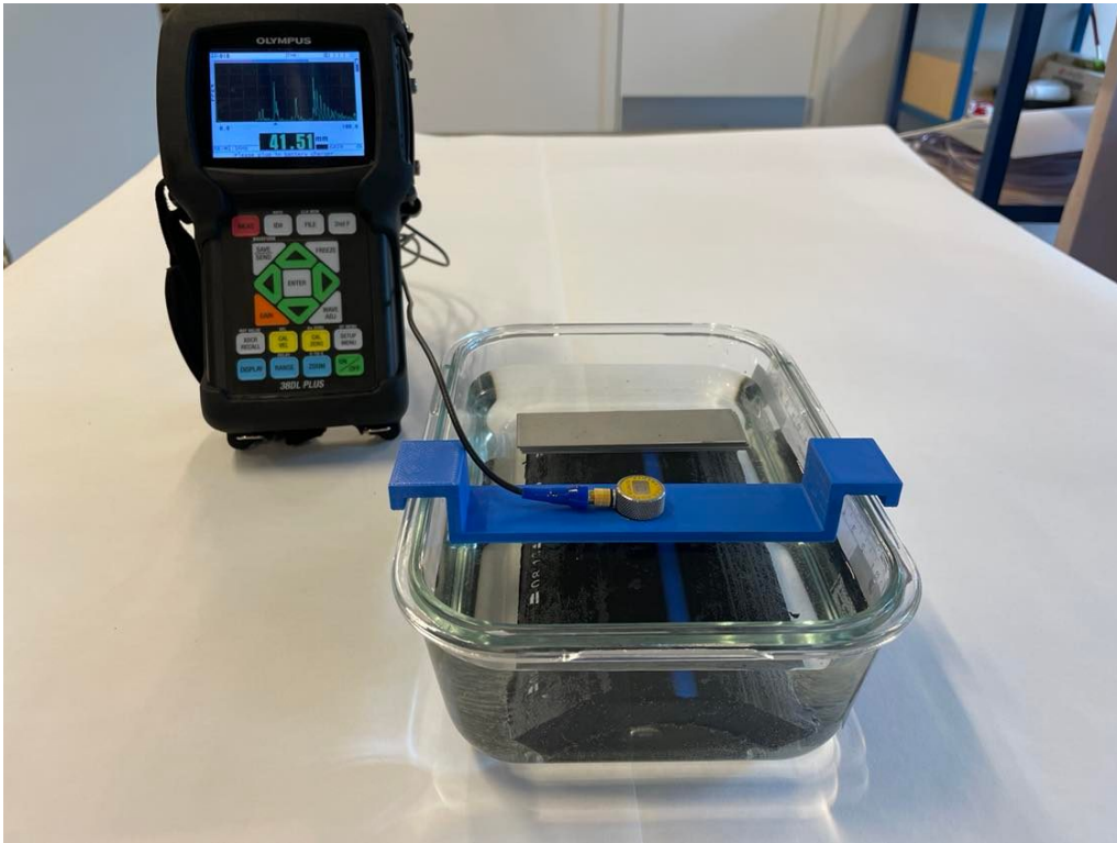
Figure 7: Test setup for immersion testing of PE pipe sample with 2.25 MHz transducer
