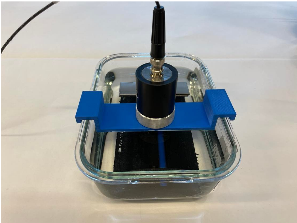
Figure 8: Test setup for immersion testing of PE pipe sample with 0.5 MHz transducer
