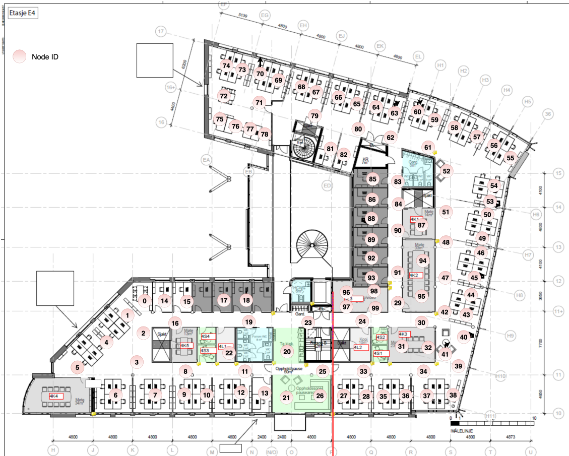
Figure 17: Large scale network office floor map - Nordic Semiconductor Trondheim. The pink dots indicate the approximate placement of each node (PCA20036 kit) in the network. The entire floor is approximately 1350 square meters.
