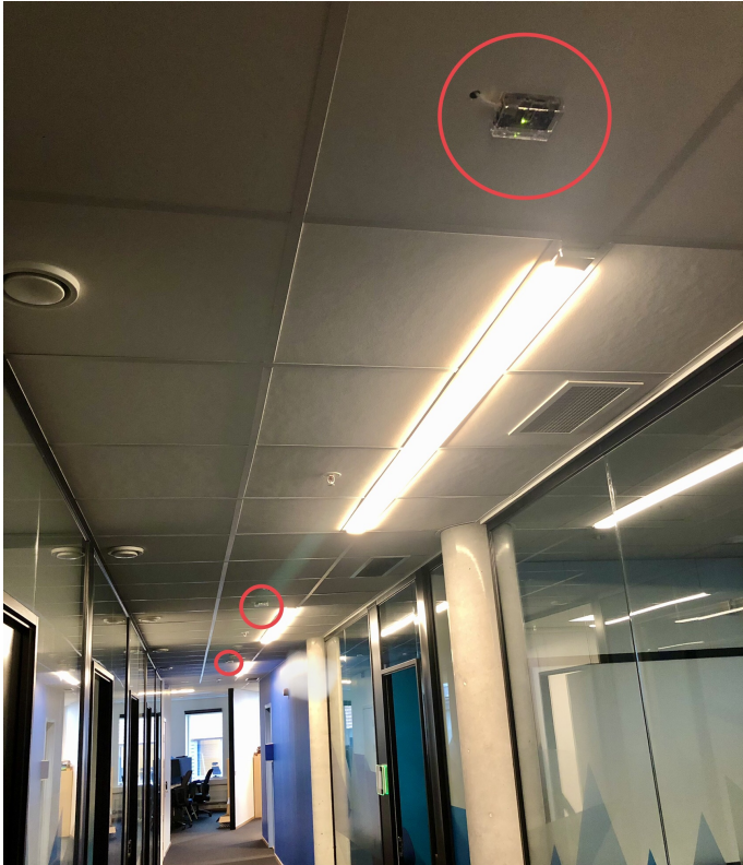
Figure 20: PCA20036 kit placement in office hallway in Trondheim. 100 kits are evenly distributed throughout the office space.
