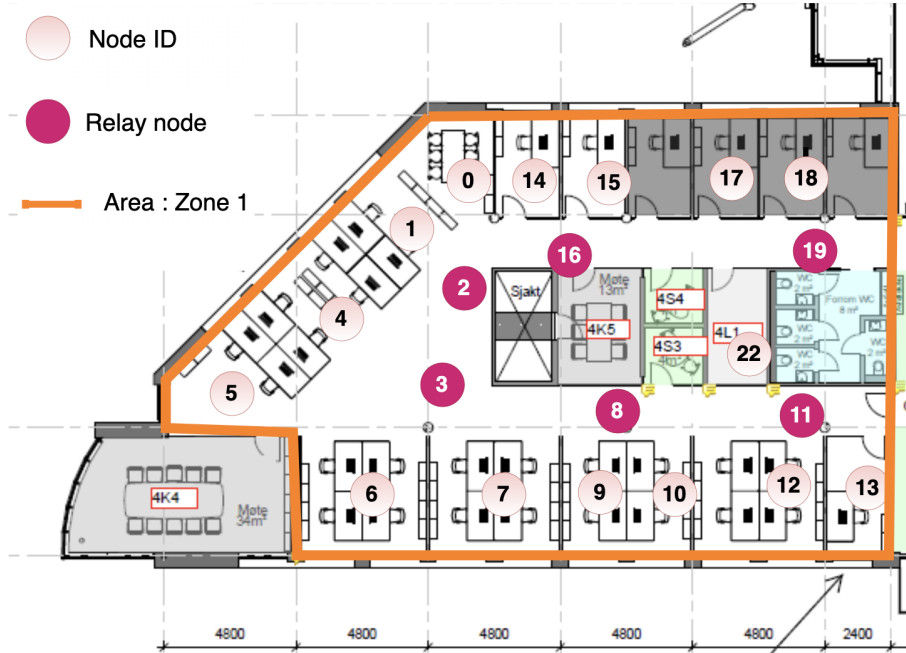
Figure 26: The isolated embedded function testing was run on a 22-node sub-portion of the large-scale 100-node network, called Zone 1.
