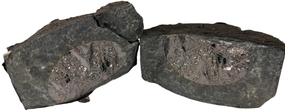
Figure 35: Product structure in experiment using \text{CaF}_2 in pre-fused slag and stoichiometric Aluminium as Reductant
