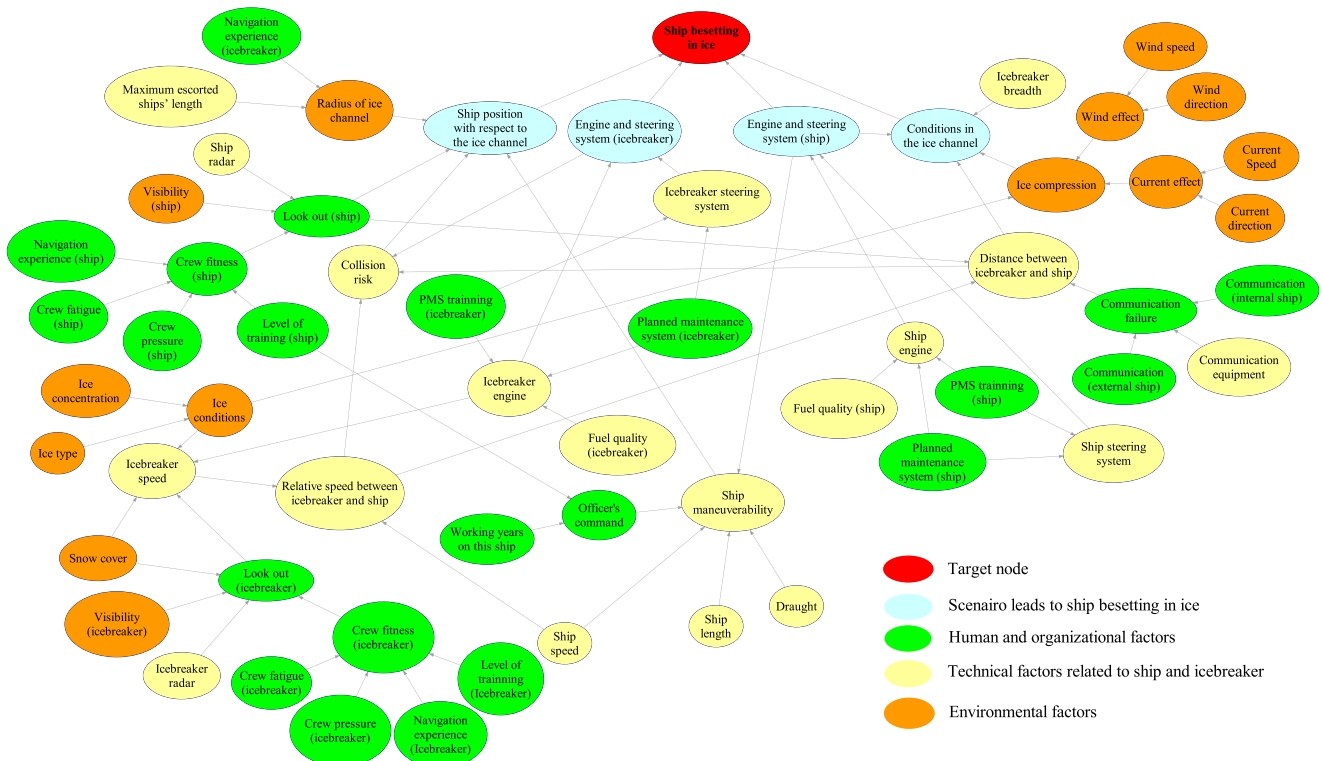
Fig. 3. Proposed BN for ship besetting in ice in convoy operations.
