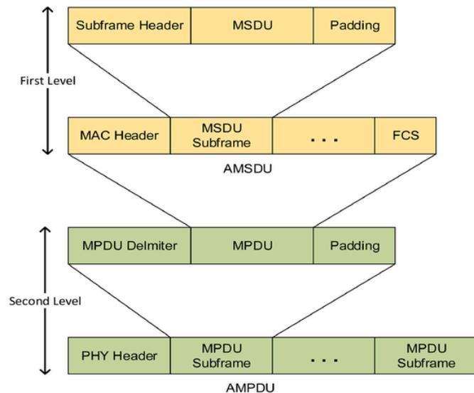
Fig. 7. Two level of frame aggregation.
