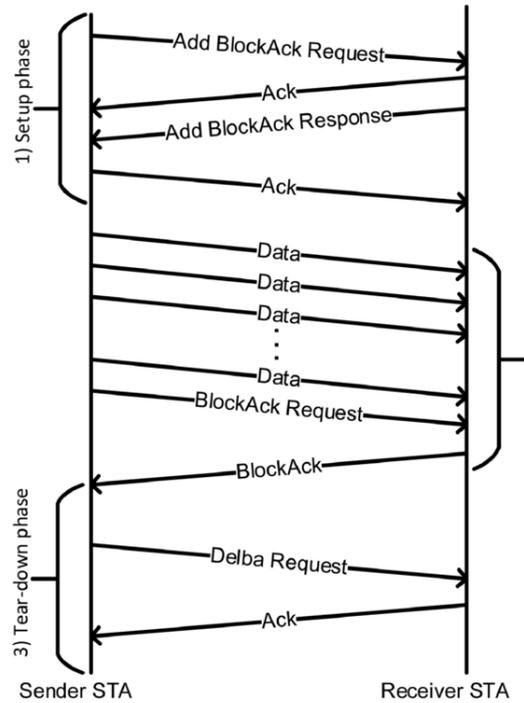
Fig. 8. IEEE 8902.11 (EDCA) BlockAck Mechanism.
