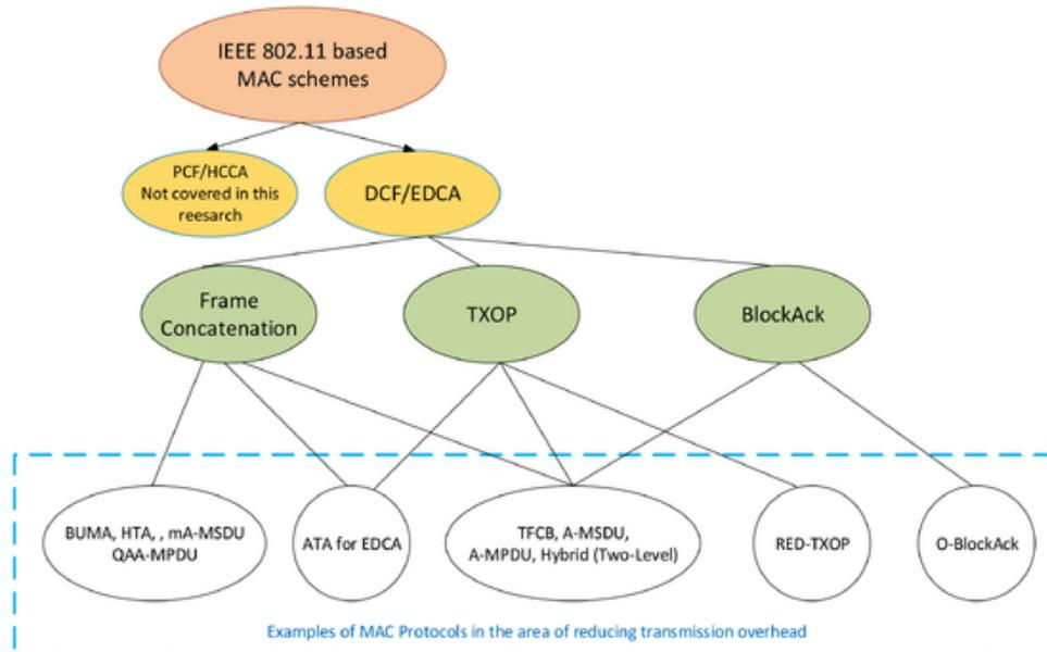
Fig. 13. Approaches used in the design of wireless MAC protocols to reduce transmission overhead.
