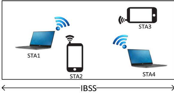
Fig. 4. A typical 802.11 wireless ad-hoc network with four STAs.
