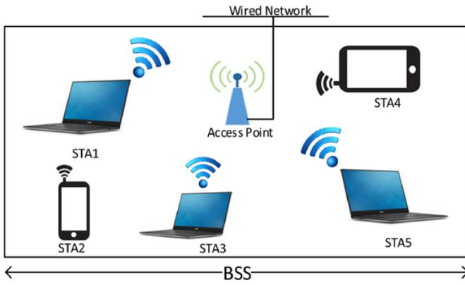
Fig. 3. A typical 802.11 wireless infrastructure network with five STAs.
